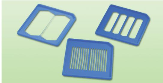
**Figure 2: More flexibility with different sample loading options.** For projects in which higher numbers of samples are needed, with fewer reads per sample, a series of gaskets are provided. These provide physical barriers to divide the PicoTiterPlate device into smaller segments, facilitating the loading of 2 to 16 samples onto one PicoTiterPlate device.
